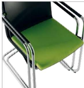
**183/3** The cantilever's stacking capability is an integral part of the design. The classy three-dimensional curve of the frame permits stacking of up to five chairs. The v-shaped side extensions of the seat shell centre the stack and the completely smooth underside of the seat shell prevents pressure marks in the seat- and backrest-upholstery.
